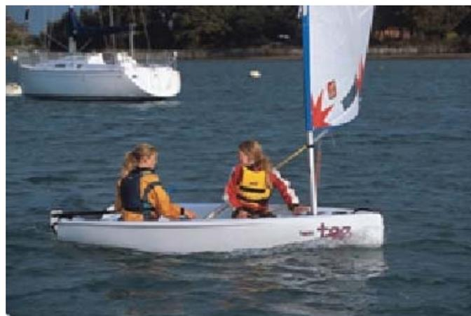
The Taz is basically a new design and it is thought that it will supersede the Topper and Optimist as the ideal training boat over the next few years. It has a moulded polyethylene hull that is reputed to be unsinkable and virtually indestructible. It should hopefully withstand any knocks and bumps received in the river and will require very little maintenance.
