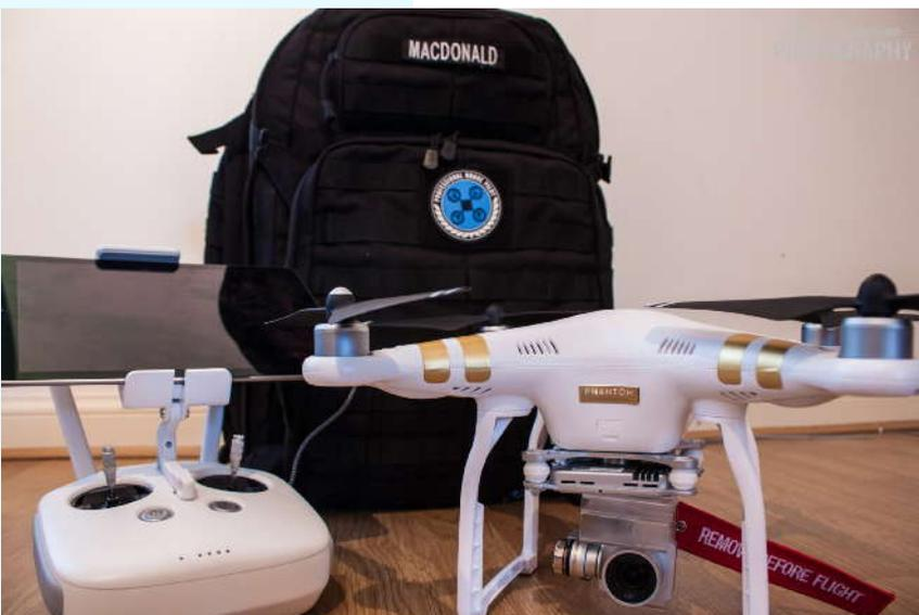
The operator has a controller and an iPad, so you can see what the drone sees, how far the drone is from you, what speed it is traveling at, its height and a map of your location.
