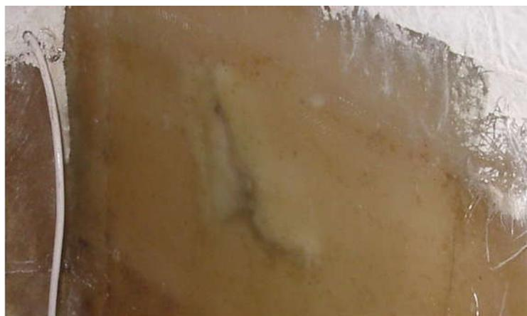
So that was the easy bit, now for the outside. I chiselled off the crazed gelcoat, and roughed up the mat. Then I mixed the gelcoat and painted it on in layers. I think that's where I went wrong. Gelcoat does not go on like paint, and nothing would give a smooth surface. If you see the state of my dinghy you will also appreciate the difficulty of working while afloat.
