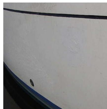
Main lesson learned: apply gelcoat the way it is supposed to go. If I was doing it again I would use a sheet of plastic on one of those flexible chopping boards and tape it firmly to the side once I had applied the gelcoat. It would need careful estimation of how much to apply. A professional would probably cut out the hole and do the repair right through from the outside in, but I was not prepared to carry out an assault like that on my boat without the confidence of knowing what I was doing.
