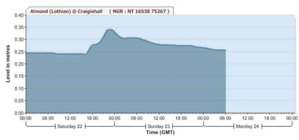
The current river level is also shown on a tide gauge type diagram. The latter shows the current level against a background of 3 river states (low, normal and high), with normal shown as between 0.25m and 3.00 metres. However, in our experience spate conditions start when the river level gets to about 1.5m. This can happen in just a few hours during periods of heavy rain.
